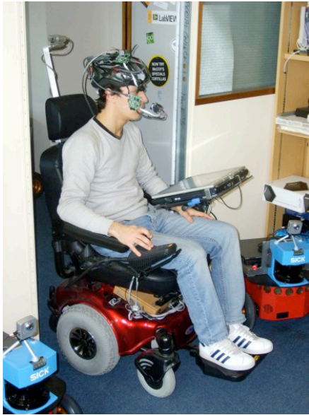
Figure 1: An example setup at Imperial's assistive robotics laboratory; human desired commands are sent through the joystick to the shared control system on a tablet PC, which estimates (through the wheelchair's cameras and laser scanners) whether the resulting action will have the intended effect, and be safe for the user, and alters the commands appropriately.
