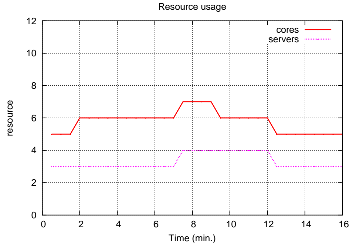
Figure 5.21: Resources used by the application over time in case of a “wonky” server
