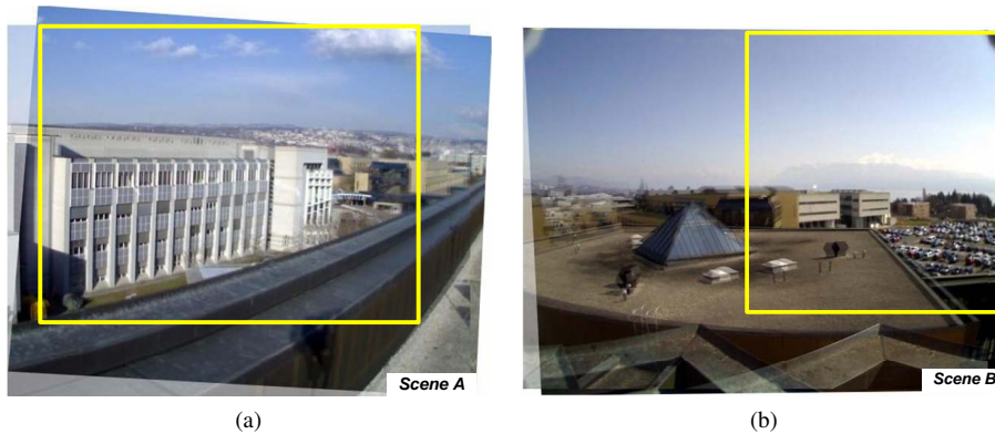
Fig. 3. Correspondence mapping using homography geometry of stereo-view images from datasets Scene A and Scene B. The registered right view is overlaid on left view. The yellow frame labels the area that is well registered.
