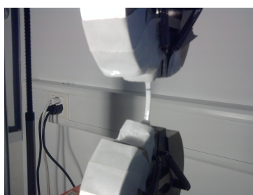
Figure 2.11: Set up of the hydrogel in the Instron machine
