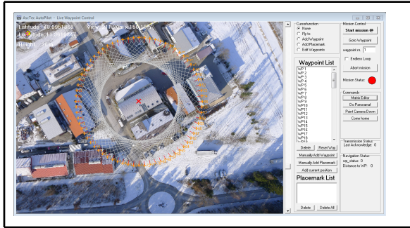
Figure 1: Flight plan of the AscTec Falcon 8
