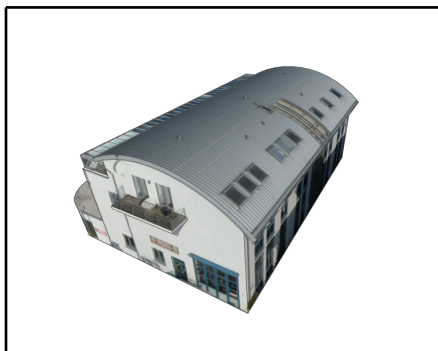
Figure 4: Refined extracted building models in Sketchup
