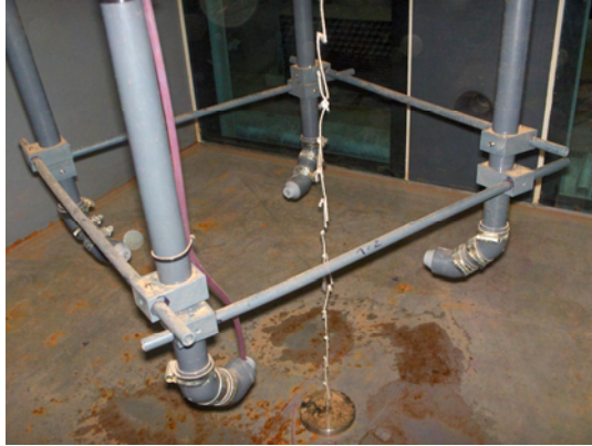
Figure 3.6 Circular jet configuration. The rigid pipes are held in a frame, avoiding flow induced vibration and therefore maintaining the exact nozzle position during the experimental run.
