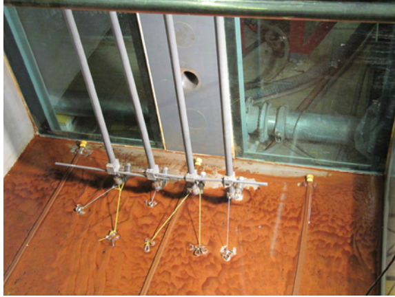
Figure 3.20 Linear jet arrangement with four jets pointing to the front wall after an experiment.
