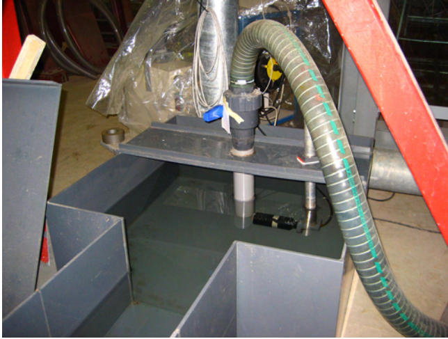
Figure 3.4 Photograph of the turbidity sensor position within the energy dissipating basin relative to the submerged jet restituting the evacuated water sediment mixture.
