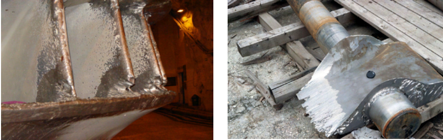
Figure 1.11 a) Damaged turbine runner and b) damaged guide vane in Nathpa Jhakri (India) (courtesy of Prof. H.-E. Minor)
