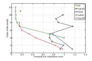
Fig. 2. Order of the identified model as a function of the normalized validation error for NucID, N4SID, PEM and FP.
