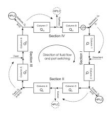
Fig. 1. Scheme of an SMB unit. The dashed lines indicate the inlet/outlet positions after the first switch. The measurements are taken by the HPLC in the extract and raffinate ports.
