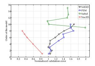
Fig. 3. Order of the identified model as a function of the normalized validation error for NucID, N4SID, PEM and Subid identified models from structured missing data.
