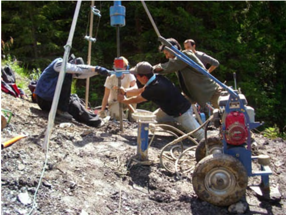
Figure 4.6: Photograph of the tripod hammer rig used on the Pont Bourquin landslide, June 2009.
