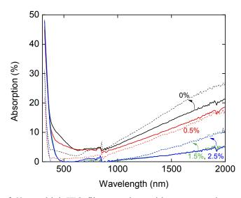
Figure 8: Absorption of 60 nm thick ITO films on glass with respect to the oxygen content in the sputtering plasma. The shown films are sputtered from the 95/5 target, the other target compositions show similar behaviour. Full and dashed lines represent films before and after annealing, respectively.
