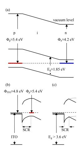
Figure 2: Schematic band diagram of the ideal p-i-n junction (upper panel). The lower panels illustrate the formation of a Schottky barrier between the p-layer and the ITO front contact. Diagram b) illustrates the space charge region (SCR) of a partially depleted thick p-layer, diagram c) shows the situation of a realistic cell with thin p-layer; the i-layer is connected to the curved part of the completely depleted p-layer, thereby reducing the attainable built in voltage.
