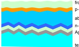
front contact p-layer absorber layer n-layer Ag-ZnO back contact
