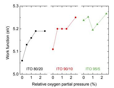
Figure 3: Work function variation of TCO films with respect to oxygen in the sputtering plasma
