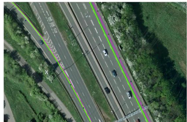
Figure 9: GPS track (green), GPS+EGNOS track (magenta) and High Accuracy Reference (points)
