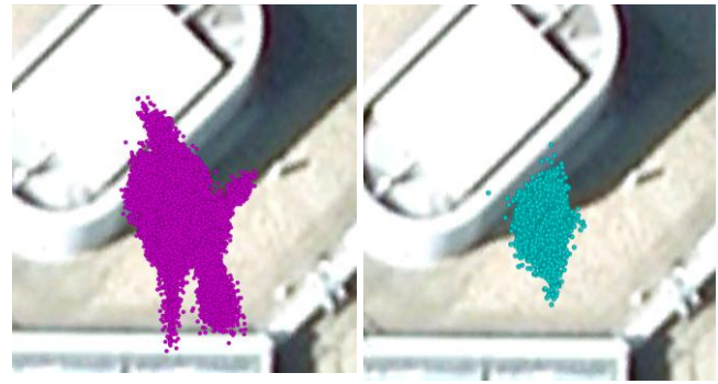
Figure 8: Reference station position estimates using a standard GPS solution (left) and with EGNOS corrections applied (right)
