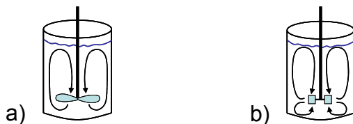
Figure 1 a) Axial and b) radial impeller type and their typical flow pattern
