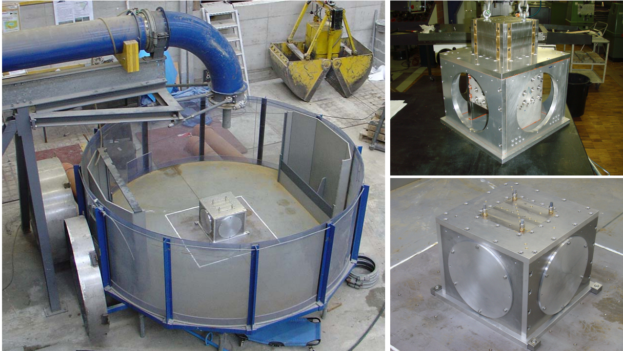
Figure 2: Left: Measurement box and highly instrumented block insert into the cylindrical basin which simulates the plunge pool. Right top: Highly instrumented block is being inserted into the centre cavity of the measurement box. Right bottom: Highly instrumented block is fully installed inside the measurement box.
