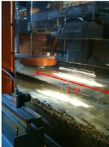
Fig. 6 The camera with a light sheet upstream of the ADVP
