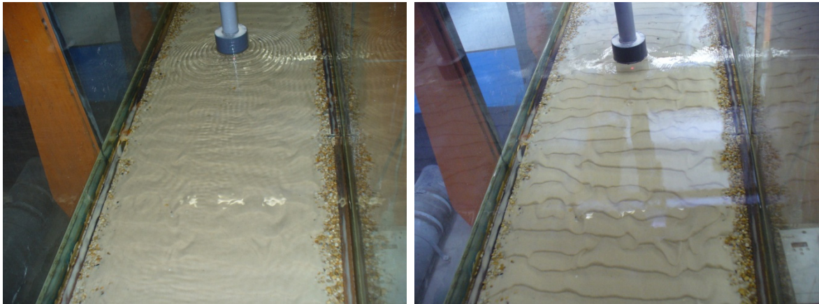
Fig. 7. The laser instrument on top of the water surface a) measurement of zero level b) measurement of ripple dimensions
