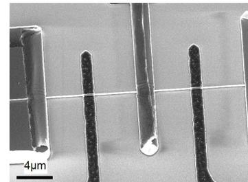
Figure 5. Inverter made with two parallel polysilicon gates and NiSi contacts.
