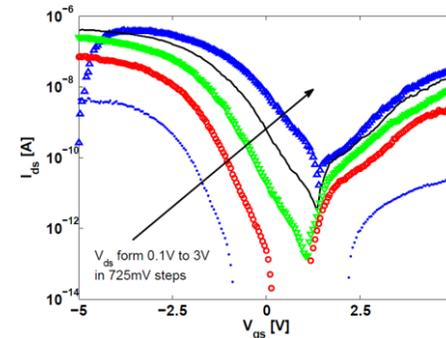
Figure 3.  $I_{ds}$ - $V_{gs}$  curve of a FET with 1  $\mu\text{m}$  long LPCVD polysilicon gate obtained by dry etching.
