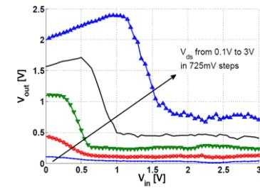
Figure 6.  $V_{out}$ - $V_{in}$  transfer characteristic of a polysilicon inverter.
