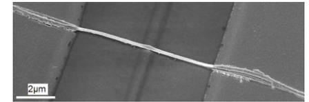
Figure 2. Si NW transistor with 150 nm x 70 nm channel cross-section and 700 nm stenciled Al gate.
