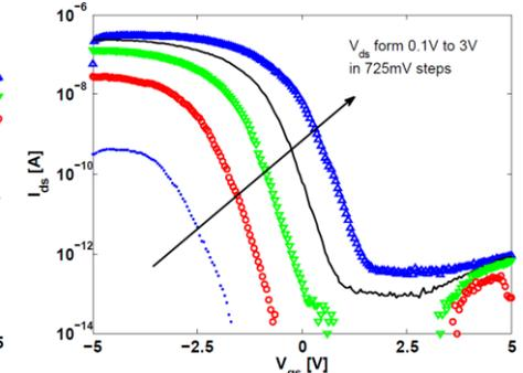
Figure 4.  $I_{ds}$ - $V_{gs}$  curve of a FET with 1  $\mu\text{m}$  long PVD Al gate deposited through a stencil.
