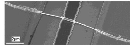
Figure 1. Si NW transistor with 100 nm x 70 nm channel cross-section and 2  $\mu\text{m}$  polysilicon gate.
