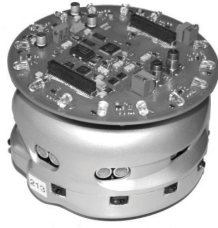
Fig. 5. The Khepera III robot with a relative range and bearing module. The board is composed of a ring of 16 infrared LEDs.
