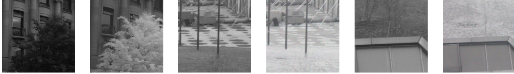
Fig. 4. Gradient reversal: differing material reflectances can reverse the direction of gradients by 180° between RGB and NIR.
