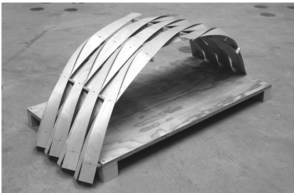
Fig. 11: Prototype of the fourth variant. The exterior layer is rotated around a central, vertical axis.
