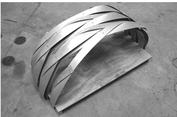
Fig. 7: Prototype of the second variant with interlaced layers.
