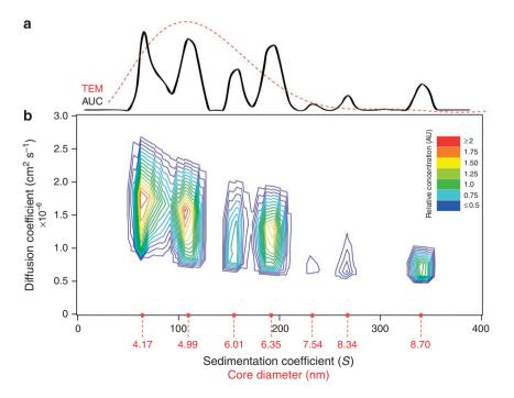
**Figure 4 | 2D AUC distribution of polydisperse gold nanoparticles. (a)** The integrated 1D distribution of sedimentation coefficients taken over all diffusion coefficients and the overlaid particle size distribution by TEM, to illustrate the increase in resolution by AUC. (b) The sedimentation and diffusion coefficient distributions for the polydisperse NP sample.
