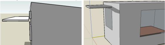
• Similarly, the easiest way to make louvers is to push/pull the part of the window between the louvers, as shown below (left: SketchUp model, right: rendering).
