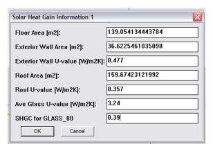
The second popup box for solar gains will ask for heat gain, ventilation, occupancy, and operational information. These are meant to be ballpark numbers; again, refer to the appendix for some suggested default values based on building type. All values for solar gains should be given in SI units.
