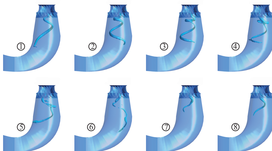
Figure 12.5: Two phase simulation (TPS) of the vortex rope precession with the SAS-SST turbulence model
