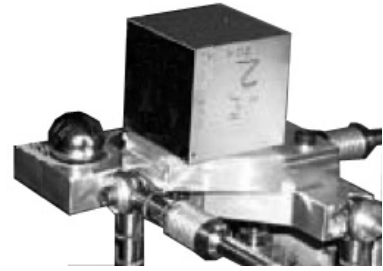
Figure 2.6: The end-effector of the Sigma6 with the mirror cube and the sphere..
