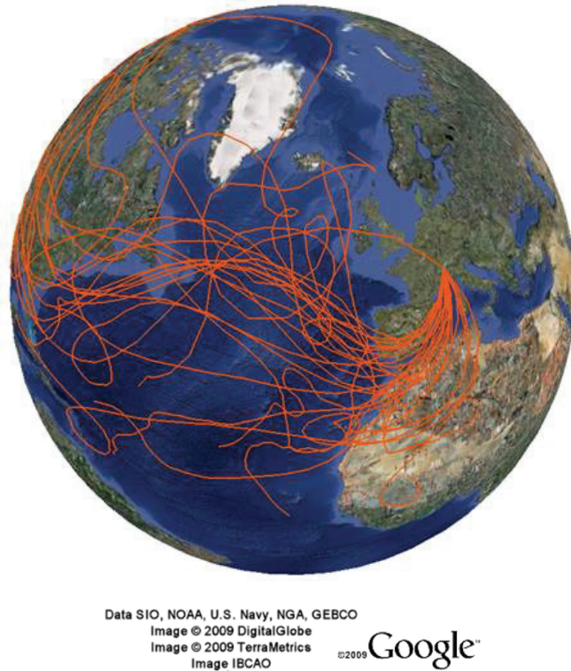
Figure 4.1 Inverse air masses trajectories at 500 hPa, corresponding to rain days with more than 100 mm at Binn station (from García Hernández et al., 2009e)
