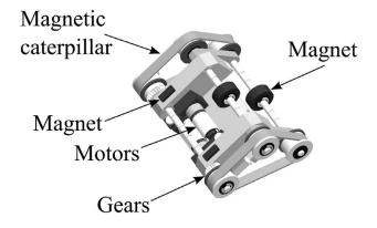
Fig. 11. 3D view of the robot.
