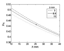
Fig. 5. Minimum  $\mu_A$  required for no slipping with  $M_A = 2.5$  N, for varying h, with three different values of b.
