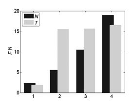
Fig. 13. Force N to lift the robot and the tangential force T to drag the robot on nonmagnetic stainless steel (a), on ferromagnetic smooth iron with low caterpillar tension (b), medium tension (c), and high tension (d).
