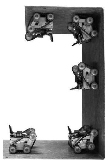
Fig. 15. The robot moving from floor to ceiling.
