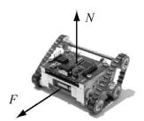
Fig. 12. The robot with adhesion and friction forces.
