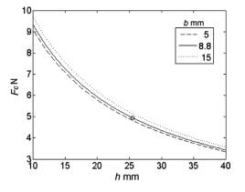
Fig. 3.  $F_C$  for  $F_A = 0$  with varying parameter *h*, the height of the front wheel *A* for three values of *b*, the horizontal distance between *A* and *B*. The circle represents the prototype robot dimensions ( $h_0$  and  $b_0$ ).
