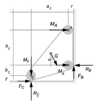
Fig. 6. Forces for inner plane transition phase 2.
