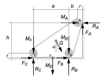
Fig. 2. Forces representation for inner plane transition in phase 1. We add the following friction relations:
