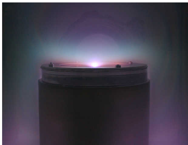
Figure 3.30: Hollow cathode, aluminium electrode, 430 Watts RF power, argon.
