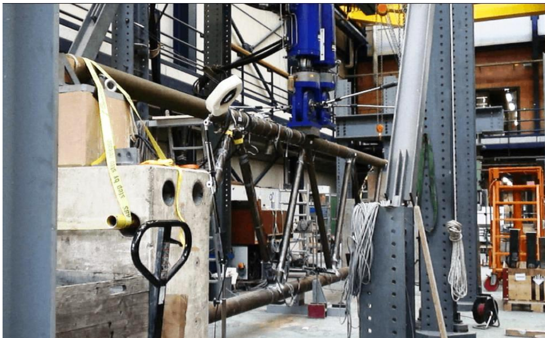
Figure 6.4: Photo of specimen S6 during the fatigue test.
