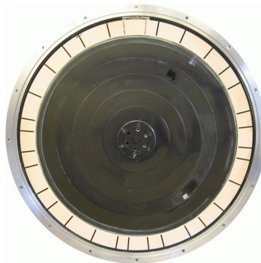
Figure 5.15: The rotating chopper disc with its 32 slits (Spallation Neutron Source SINQ, 2009).
