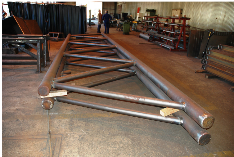
(c) Photo of the two truss beams at the steel factory
