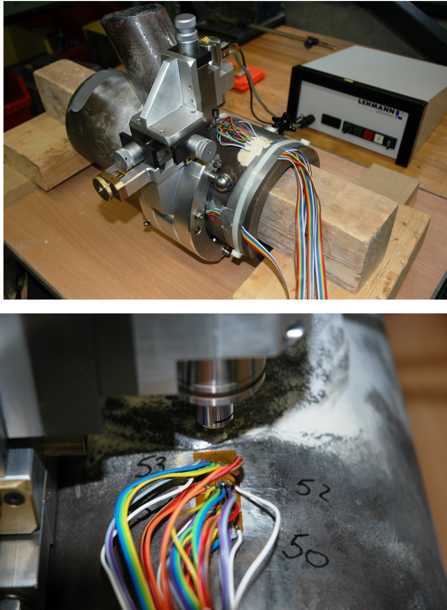
Figure 5.5: Hole-drilling device installed and ready to drill the hole.
