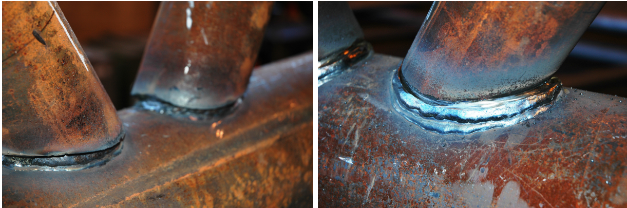
(a) The weld geometry after two passes.
