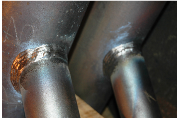
Figure 6.2: Joints J4S at support position after needle peening.
