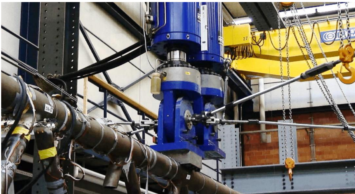
Figure 6.5: Actuator Hydrel 1200 kN for fatigue solicitation.
