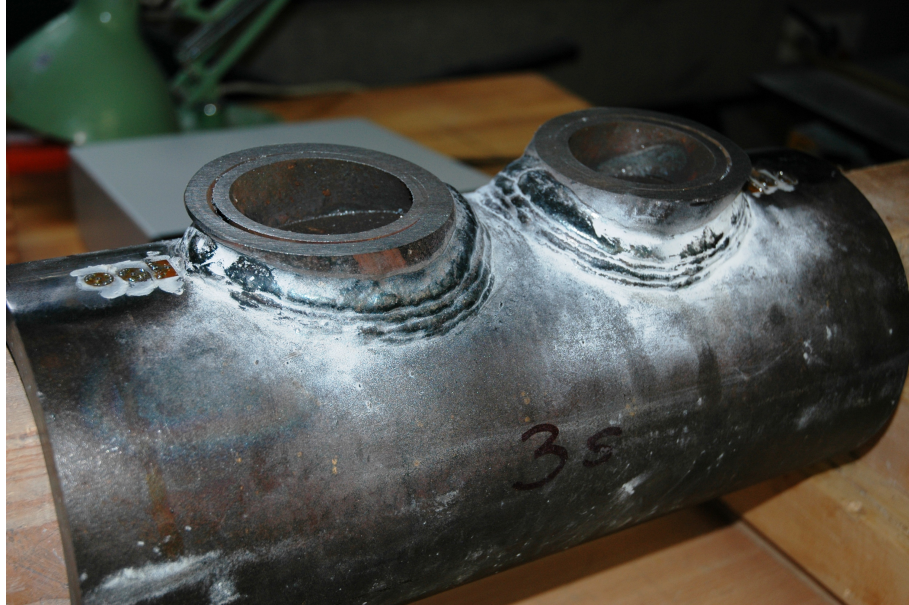
Figure 5.8: Hole-drilling rosettes glued in the crown heel area for residual strain measurements.
