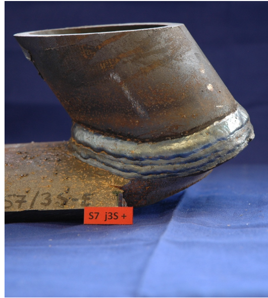
Figure 9.3: View of the real crack surface (fatigue test).
