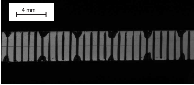
Figure 3.4: Graduation on the side of a delaminated sample.
