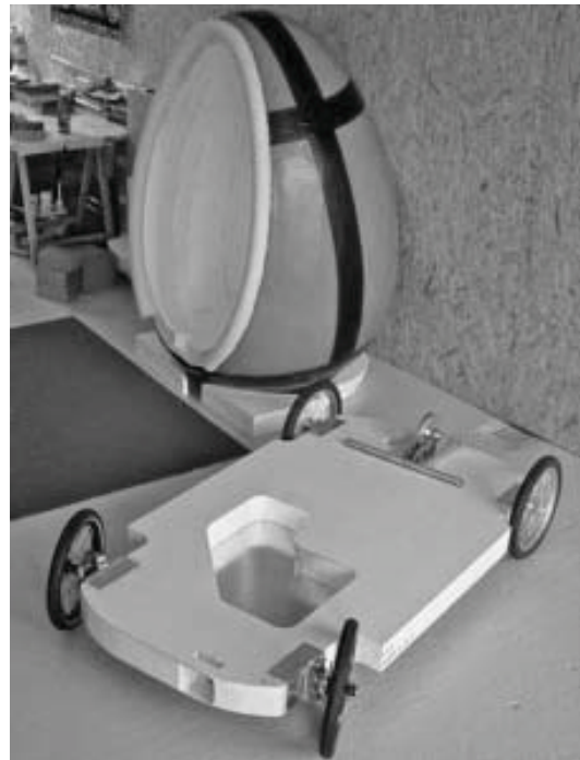
Fig.2 Unique structure of UCV, with sandwich plate for rolling platform and foam cabin in form of a large safety helmet.
