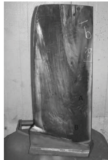
Fig. 3. Compressor's Blade damage (1 st stage)
