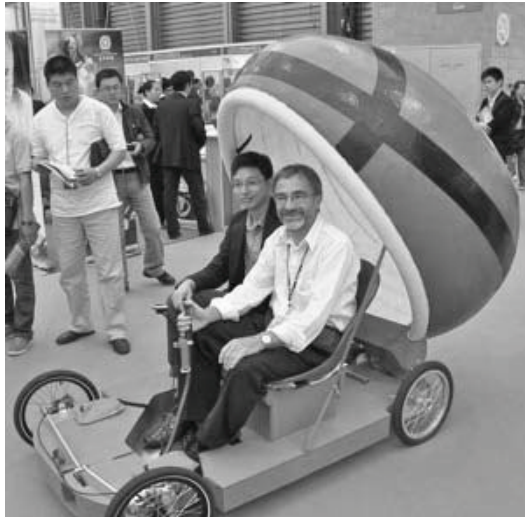
Fig.3 For access, the helmet type cabin is lifted up and swings back.
