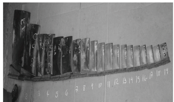
Fig. 4. Compressor's Blade damage (all stages) due to a bad fogging System Operation.
