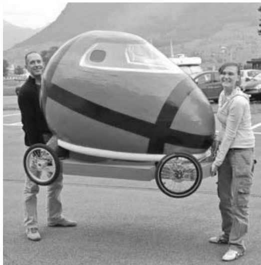
Fig.1 Unique City Vehicle UCV with weight of two electric bicycles.
