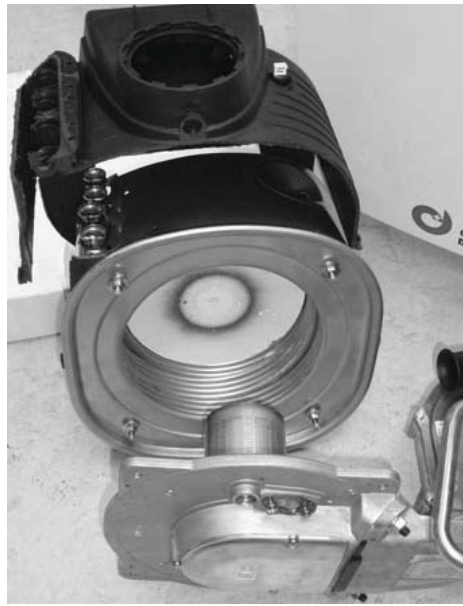
Figure 2: The disassembled heating unit with its combustor in the foreground. One can see the perforated sheet metal cylinder.
