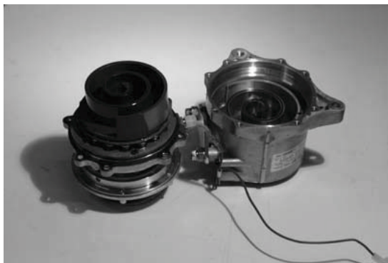
Figure 3: Global view of the domestic heat-pump booster compressor (opened).
