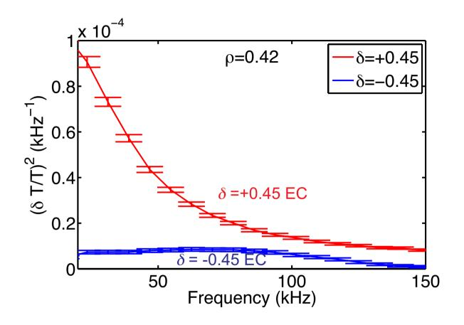
going from  $\delta$ =+0.45 to  $\delta$ =-0.45, results in a strong reduction of fluctuations; especially below 80kHz
