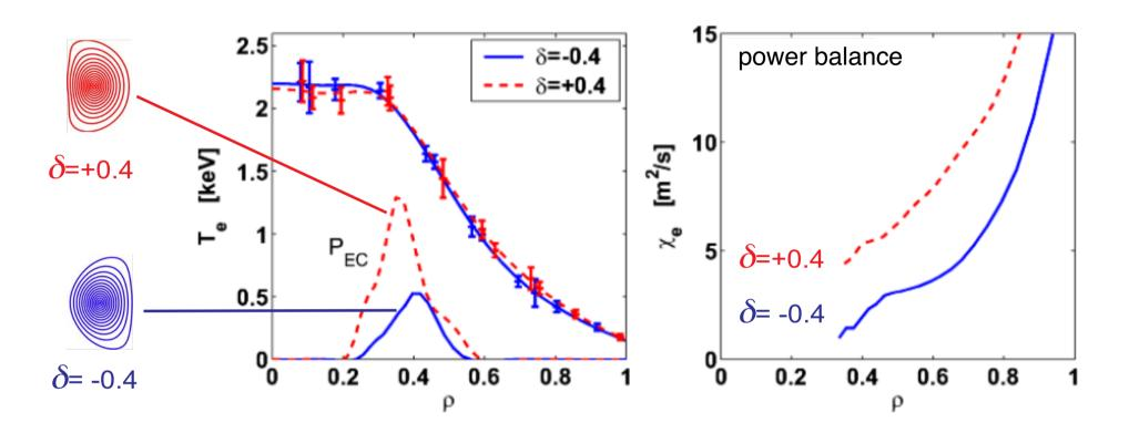
Adjusting power at each triangularity  $\delta = \pm 0.4$  to reach the same  $T_{\rm e}$ ,  $n_{\rm e}$ , (i.e. same plasma energy), and q-profiles :
