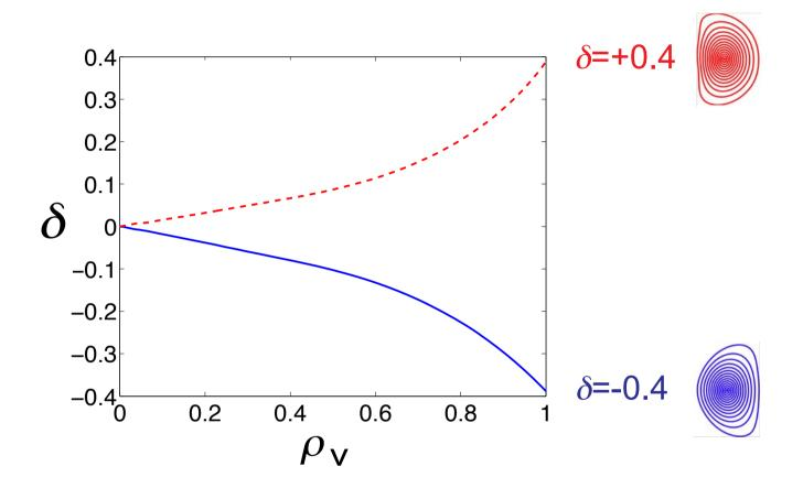
Large transport variations with  $\delta$  measured at mid-radius, but triangularity at mid-radius only represents ~25% of  $\delta_{
