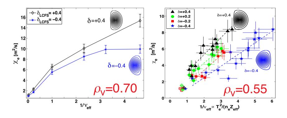
• From flux-tube calculations, triangularity effect on  $\chi_{\rm e}$  remains confined to the edge
