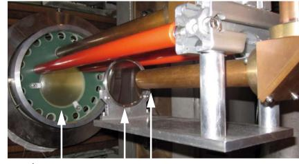
lens polarizer waveguide entrance
