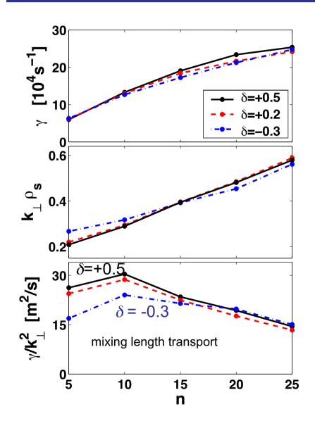
Mixing length transport estimate reduced for  $\delta < 0$ , through reduction of  $k_{\perp}$  at low n
