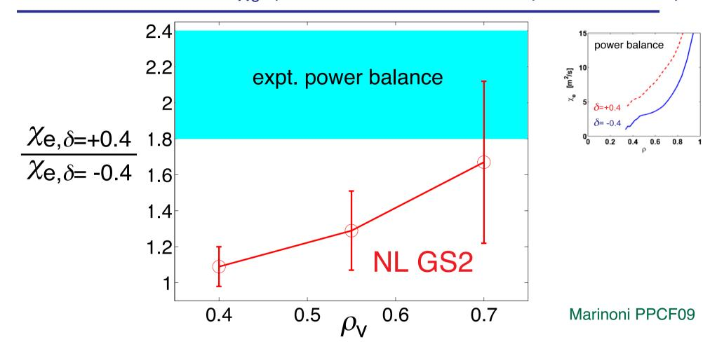
Triangularity effect on  $\chi_e$  from local GK simul. vanishes towards the centre, unlike in experiment, where the triangularity effect does penetrate
