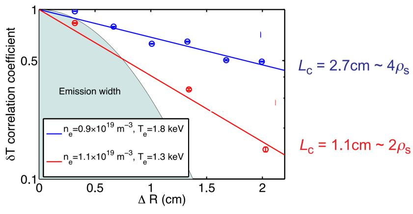
at given power,  $L_c$  very sensitive to density, which needs to be well controlled
