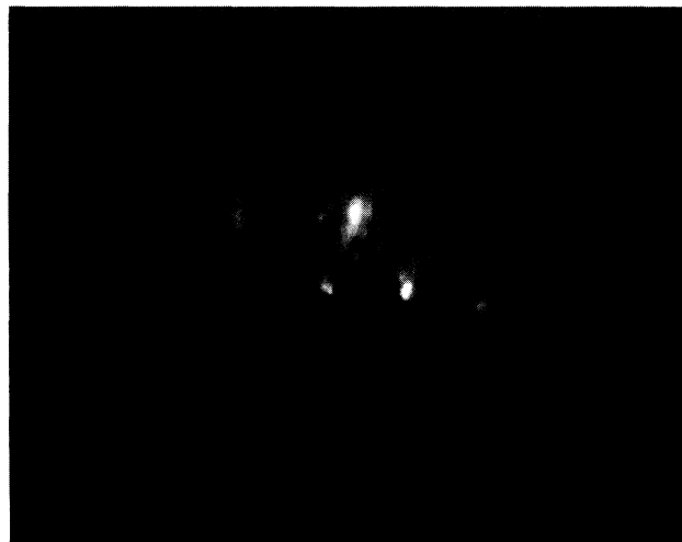
Fig. 10 Fluorescence image of a hexadecane sample containing terrylene molecules. The sample was illuminated at 574.319 nm with 25- \mu W laser power. The fluorescence light was integrated over 10 s. The diameter of the imaged sample region was estimated to about 100 \mu m.
