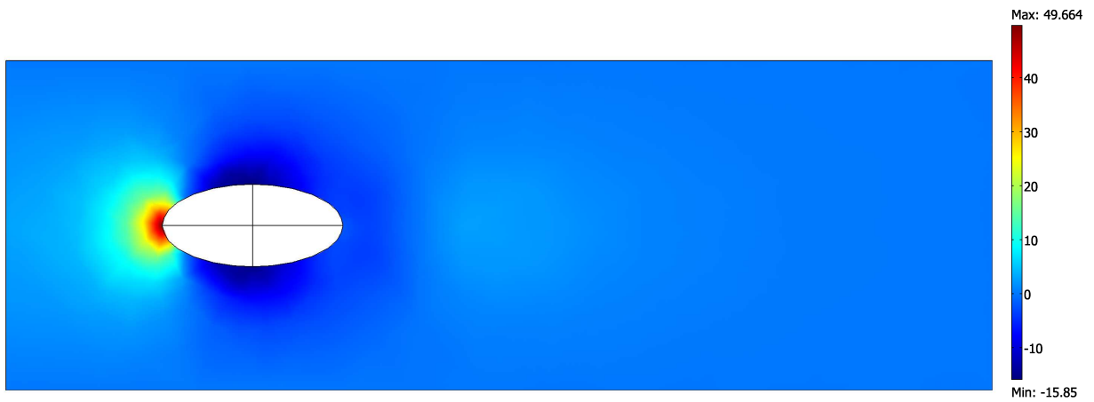
Figure 5.5: Pressure field of the initial shape of the bulb in plane XY [Pa].
