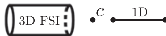
Figure 13. Geometrical multiscale coupling between a fluid–structure interaction (FSI) model and a 1D model.
