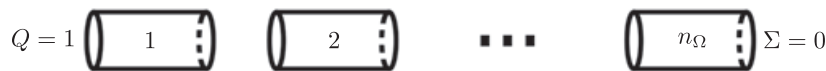
Figure 3. Serial network of n_\Omega cylinders connected by \mathcal{C} = n_\Omega - 1 couplings. On the left, we impose a unitary flow rate, whereas on the right, a no-stress Neumann boundary condition is applied.
