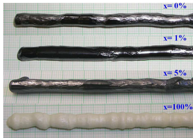
Fig. 3. As-grown single crystals of \text{Bi}(\text{Cu}_{1-x}\text{Zn}_x)_2\text{PO}_6 ( x=0\% , 1%, 5%), together with rod of \text{BiZn}_2\text{PO}_6 .
