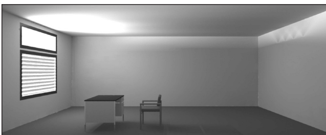
Pict. 3. Photorealistic visualization of room illuminated by standard venetian blinds in the lower facade area and a light redirecting glass in the upper facade area.
