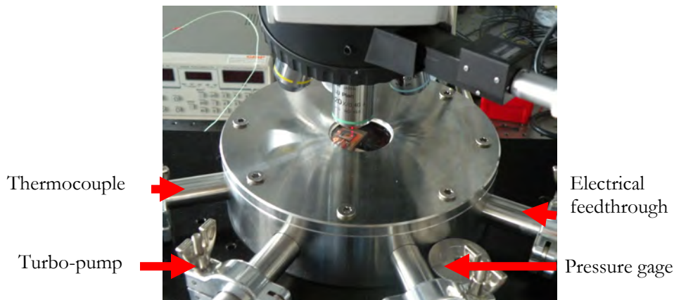
Figure 6: Close-up of the test chamber for specimen frequency measurements in a controlled environment
