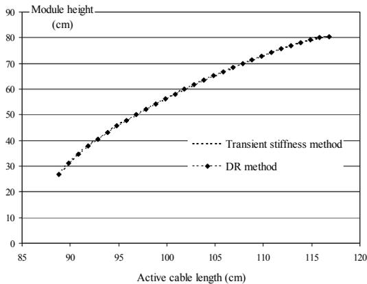
**Figure 11.** Actuation-response of the clustered tensegrity structure
