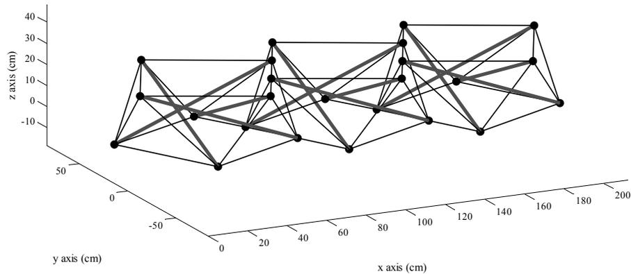
**Figure 3.** A perspective view of the tensegrity beam
