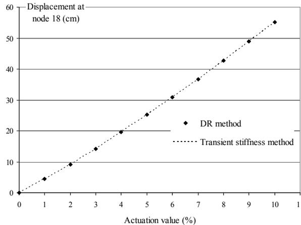
**Figure 5.** Actuation-response of the clustered tensegrity beam
