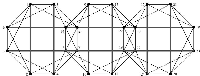
**Figure 4.** Clustered elements of the tensegrity beam
