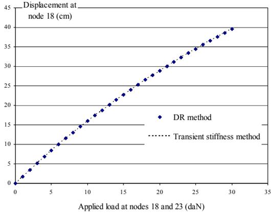
Figure 7. Load-displacement curves of the clustered tensegrity beam
