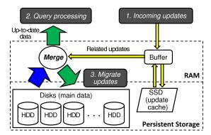
Figure 2: Framework for SSD-based differential updates.
