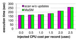
Figure 13: Range scan and MaSM performance while emulating CPU cost of query processing (10GB ranges).
