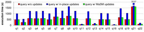
Figure 14: Replaying I/O traces of TPC-H queries on a real machine with online updates.
