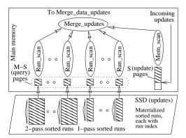
Figure 7: Illustrating MaSM algorithm using M memory.
