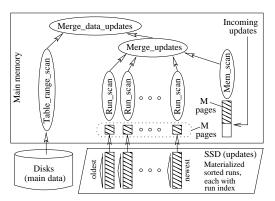
Figure 6: Illustrating the MaSM algorithm using 2M memory.
