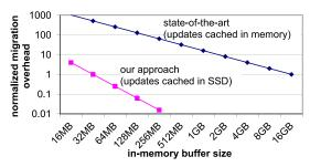
Figure 1: An analysis of migration overheads for differential updates as a function of the memory buffer size. Overhead is normalized to the prior state-of-the-art using 16GB memory.
