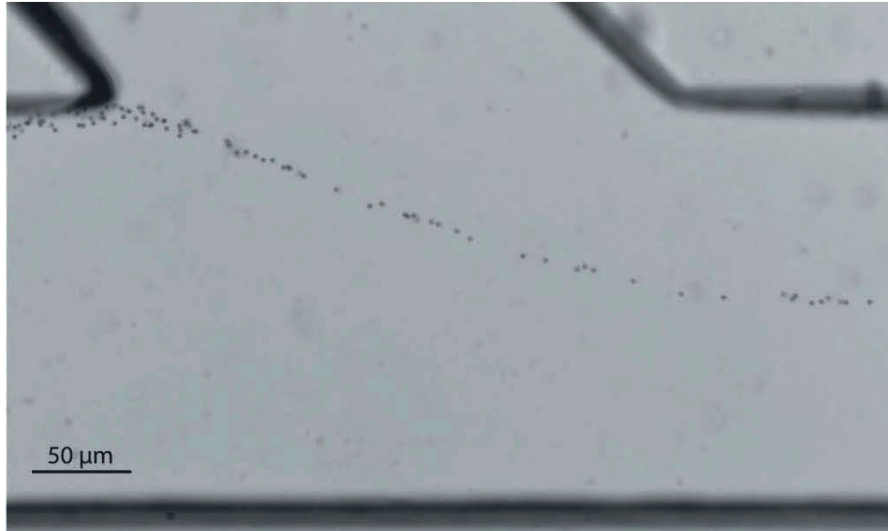
FIGURE 3: Photograph demonstrating focusing and alignment of 1\ \mu\text{m} beads during deviation and acceleration of the stream at the junction of the main and the secondary flow channels. The final bead velocity is 0.6\ \text{mm/s} .
