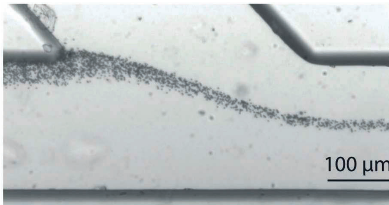
FIGURE 4: The lateral dimension of the focused stream varies as a function of the flow velocity. Reducing the maximum speed in the main channel to 0.3\ \text{mm/s} clearly results in a less confined bead stream (in this picture the number of beads in the plug is more than 400).
