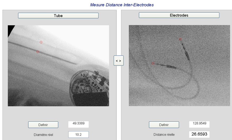
Figure 5.10: Inter-electrodes distance. X-ray of the tracheal tube (left) and of the two right atrial leads (right). Using the diameter of the tracheal tube as reference (10.2 mm) gave a distance of 26.7 mm between the two leads.
