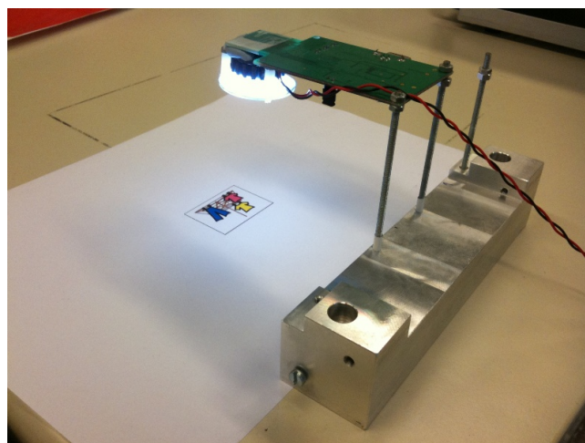
Figure 5: Camera setup with LED crown
