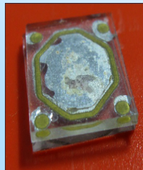
Sealed glass cell with Rb inside: the Rb looks silver in colour, hence it is not oxydized
