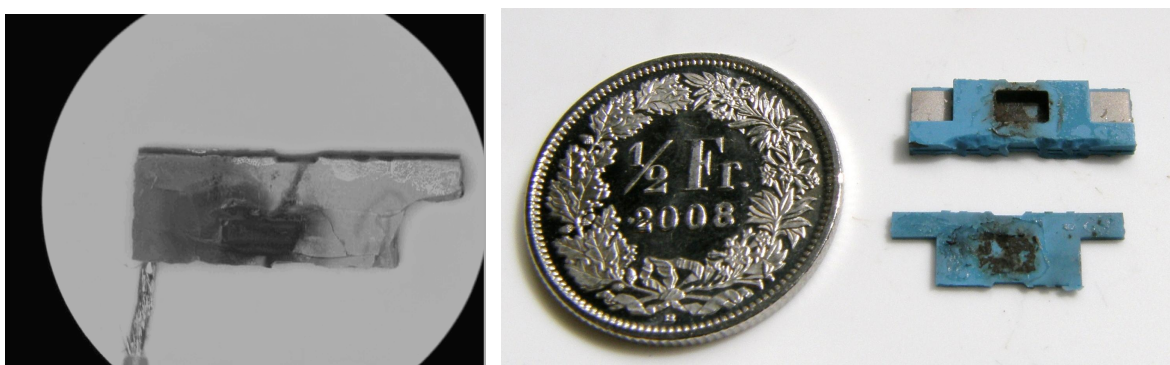
Fig. 11. A failed microthruster due to insufficient wall thickness (left) and glue bond strength (right).
