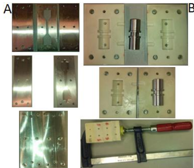
Figure1. A: Mould assembly process for the production of the shouldered test bar. B: Mould assembly process for the production of the encapsulation chamber production.
