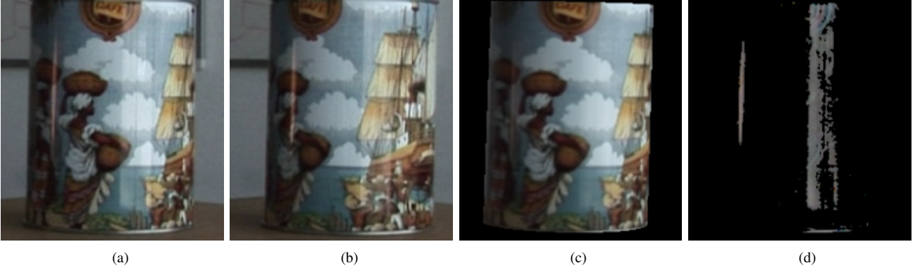
Figure 4. Estimation of texture and reflections. (a,b) First and last frame of a video sequence. (c,d) The diffuse and specular images computed as described in Section 3.2. Image (d) was gamma-corrected for clarity.
