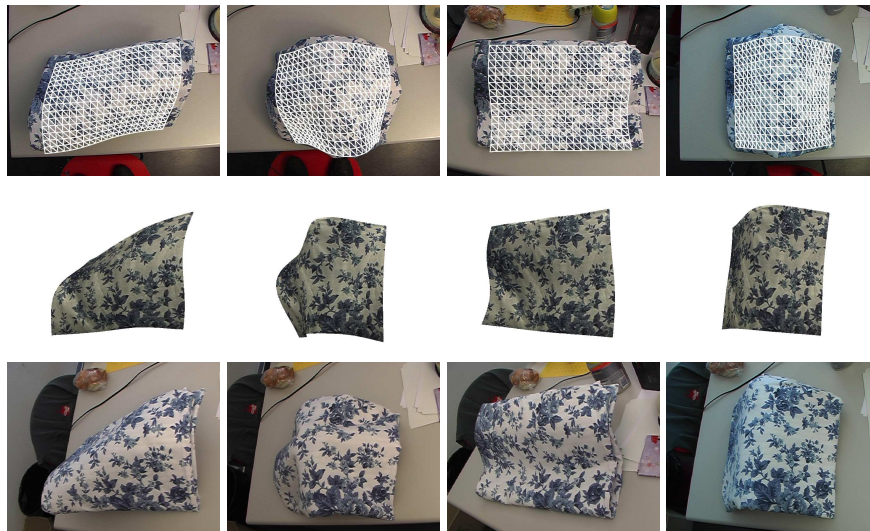
Fig. 5. 3D registration of a folded bed-sheet to an individual image given a reference configuration. Top Row: Recovered mesh overlaid on the original image. Middle Row: Synthesized textured view using the recovered shape. Bottom Row: Real side view of the sheet from similar viewpoints. Despite lighting changes, the synthetic images closely match the real ones.
