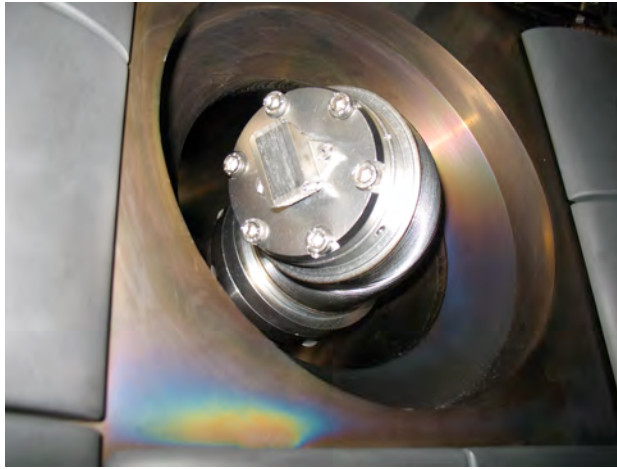
Fig. 3.3.3 View of the X-ray diagnostic head from inside the vessel. The system is rotated to a typical near-tangential viewing direction.
