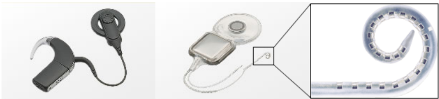
Fig. 1-11: Cochlear implant (Cochlear Nucleus 5): audio processor on the left, implant in the middle and a magnified view of the stimulation electrode on the right [11]
