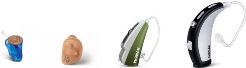
Fig. 1-8: Conventional hearing aids, from left to the right: completely in the canal device (CIC), in the canal device (ITC), micro behind the ear device (micro BTE), behind the ear device (BTE) [6]
