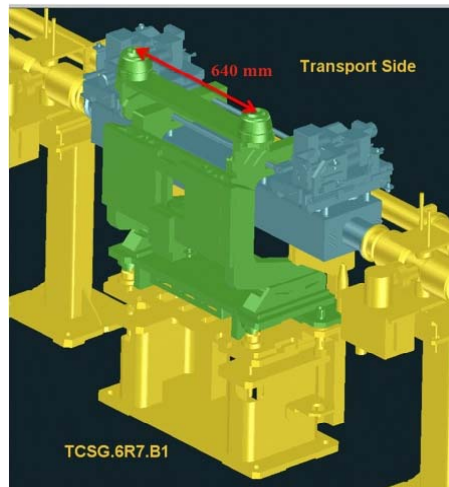
Figure 10.2: Sketch of a horizontal Phase I secondary collimator installed in the LHC tunnel. The two reference points located on the tank are used for the alignment of the collimator with respect to the upstream and downstream elements of the machine.
