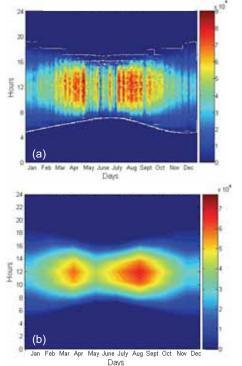
Figure 2. Temporal Maps for a North-facing façade in Sydney displaying outside vertical illuminance in lux, based on (a) five minutes intervals using DAYSIM and (b) a reduced set of 56 data points for Lightsolve
