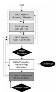
Figure 7. Flow chart illustrating the interactive optimization approach chosen for Lightsolve.
