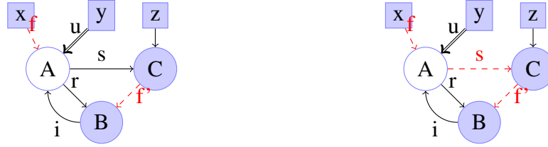
Figure 4.2: Comparing (a) external uniqueness and (b) separate uniqueness ( \Rightarrow unique reference, \rightarrow legal reference, --\rightarrow illegal reference)
